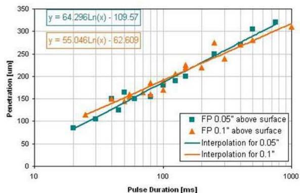
**Figure 5** Effect of pulse duration on weld penetration
