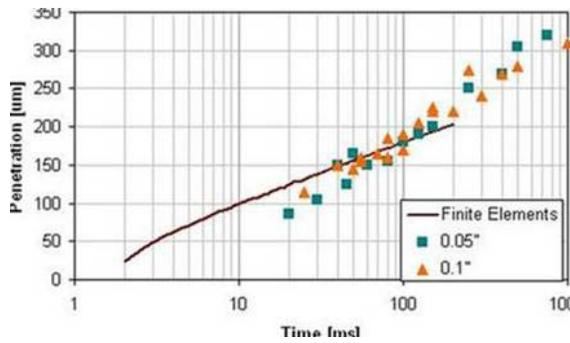
**Figure 6.** Experimental and simulated weld penetration
