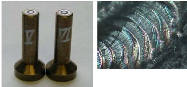
**Figure 7.** Welded Sample, with close up of the weld
