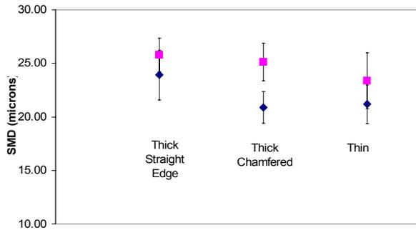
**Figure 11.** SMD for 3D 10X80+1X60 nozzle
