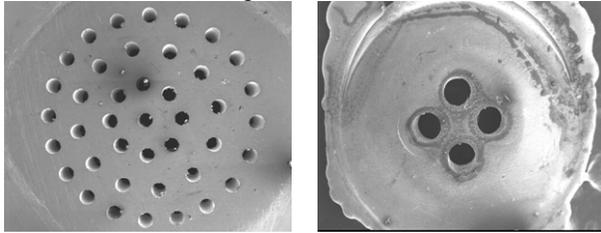
**Figure 2.** 3D 41X80 and 4X260 micro-nozzle
