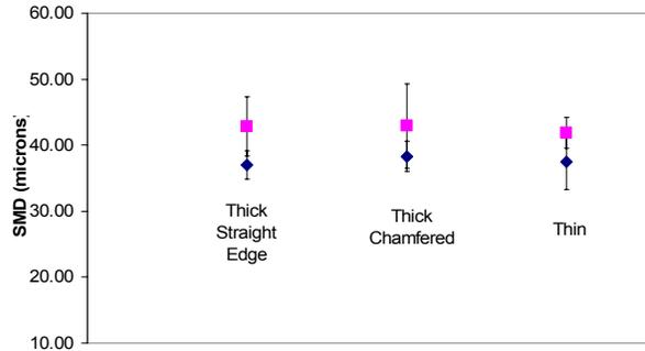
**Figure 13.** SMD for 3D 41X80 nozzle
