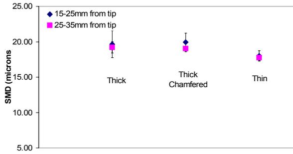
**Figure 10.** SMD for planar 40X40+1X60 nozzle
