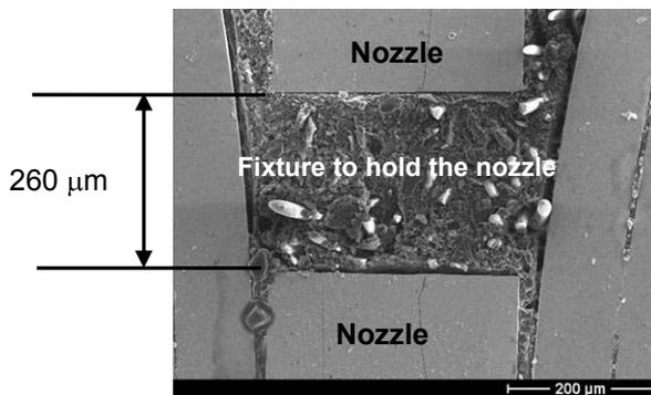
**Figure 16.** Cross section of a LIGA fabricated nozzle
