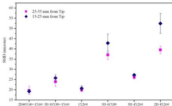
**Figure 15.** Effect of nozzle configuration with thick clamp on SMD
